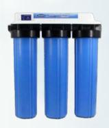
Wall mounted three stages DI water filtration system consisting of a carbon block filter and a pair of Mix Bed Filter. Produce up to 2000 litres of DI water comply to BS3031 and DIN 43 530-1 standard. Water use for topping up lead acid batteries (Conductivity less than  $30\mu$ S/cm).
